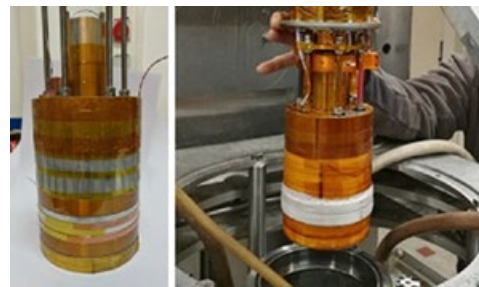
Figure 1: Pictures of the HTS mock-up insert. Left, before over-banding. Right, during its insertion into the cryostat.
