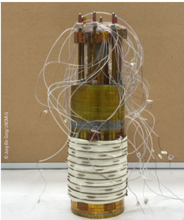
HTS insert magnet with its instrumentation wiring before mounting on the characterization probe.
