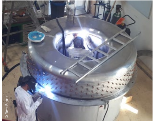
Figure 2: Closure welding of the He vessel with the superconducting coil inside requiring a strict control of the temperature to not damage the electrical insulation (contractor SDMS).
