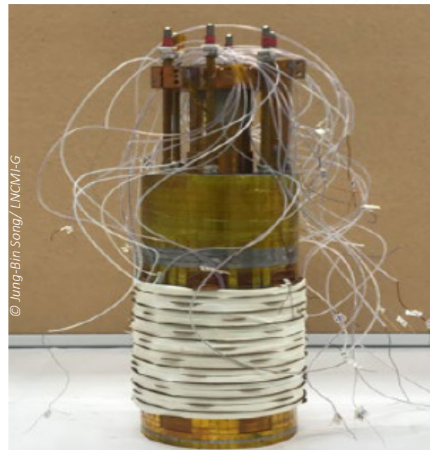
HTS insert magnet with its instrumentation wiring before mounting on the characterization probe.
