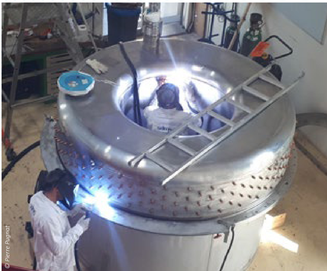
Successful insertion of the superconducting coil in the He vessel. In the most constraint part, the radial clearance is 0.4 mm.
