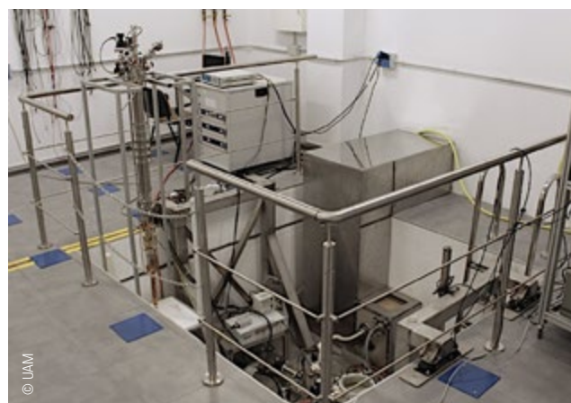
› Overall view of the 22 Tesla magnet. Magnets in the lab are located inside a pit, allowing for the use of long cryostats and for a near to zero residual magnetic field in the lab space.
