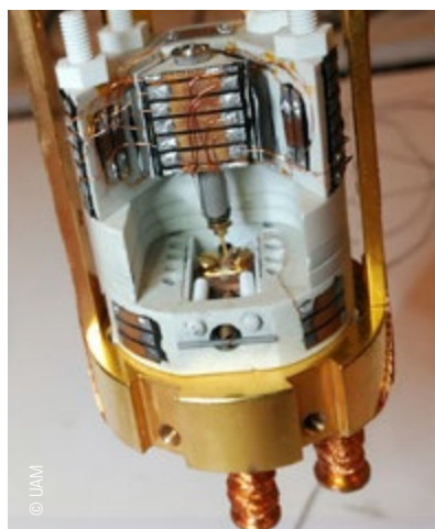
› STM head made of nonmetallic Shapal mounted on the low-temperature stage of a dilution refrigerator before insertion into a high-field magnet.
