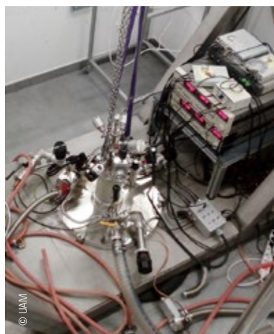
› Dilution refrigerator being inserted inside the cold 22 Tesla magnet.
