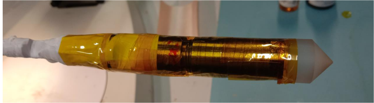
DAC for 85 T pulsed field, d = 15.3 mm, Ni-Cr-Al alloy
