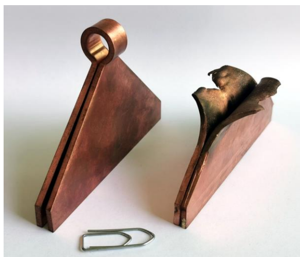
Figure 4: Single-turn coil before and after the pulse
